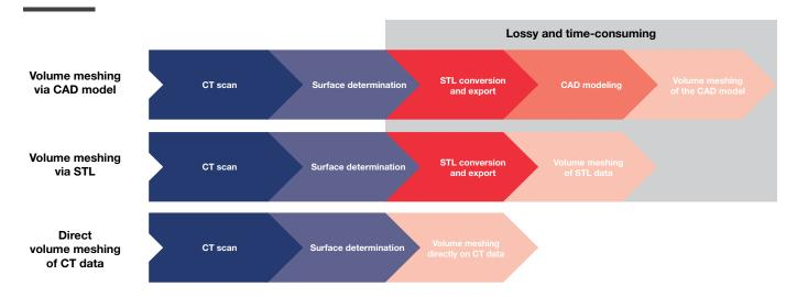
Volume Graphics software allows you to create tetrahedral volume meshes of your parts directly from the voxel data of a CT scan at the push of a button with virtually no loss of time or quality. The Volume Meshing Module for VGSTUDIO MAX can save you up to 80% of the calculation time compared to the traditional method of STL conversion with subsequent optional CAD modeling.
