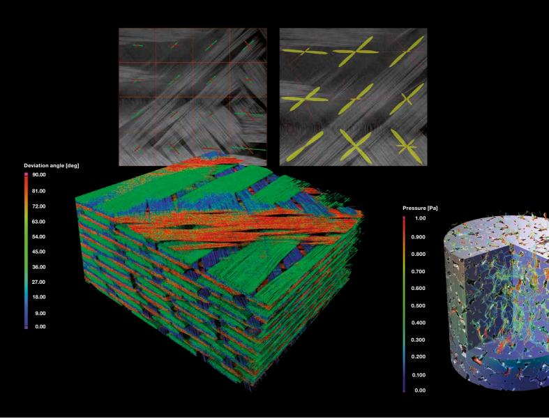
[4] Multi-layered fabric with color-coded orientations, main directions, and orientation distribution
