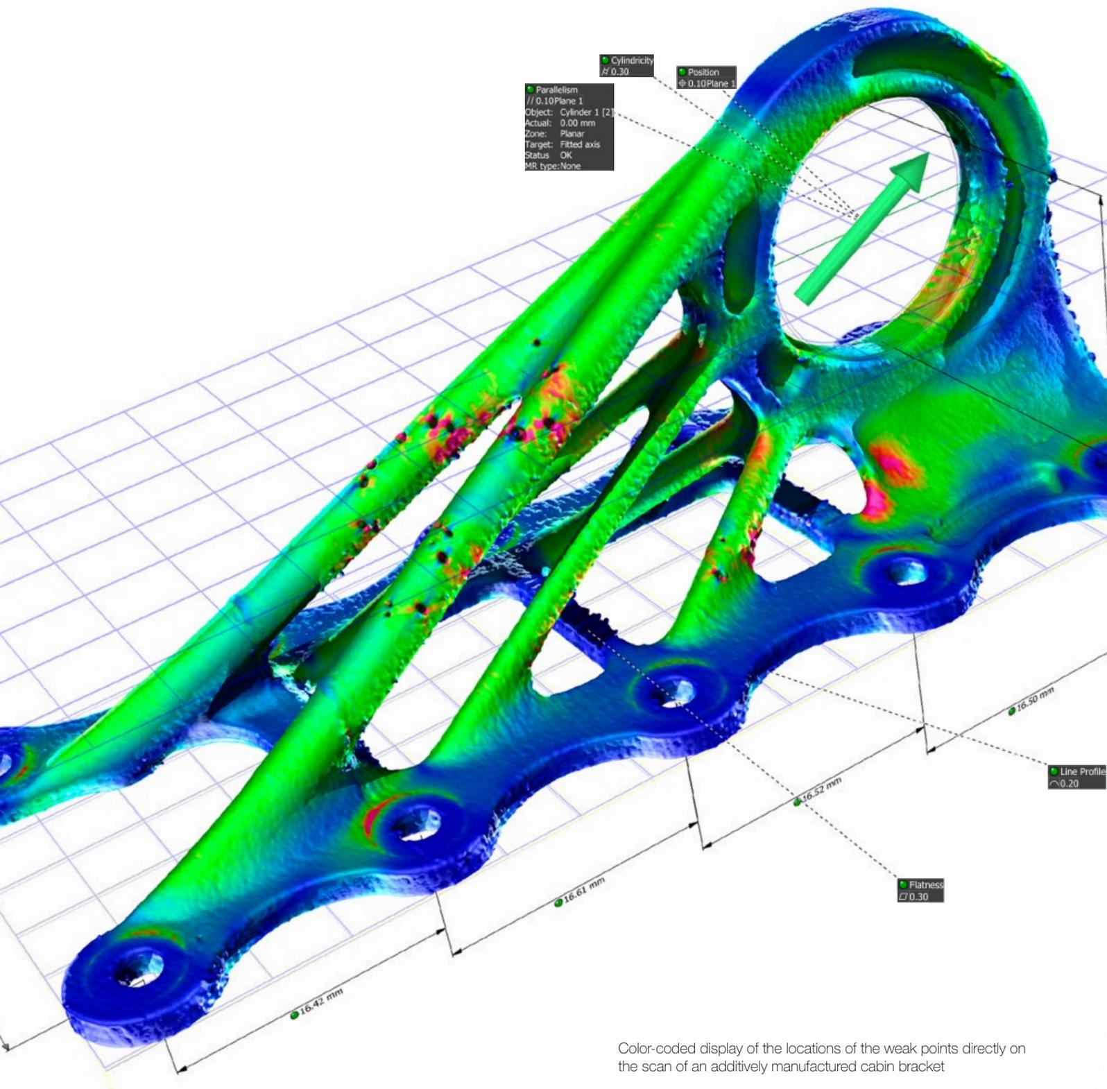
Color-coded display of the locations of the weak points directly on the scan of an additively manufactured cabin bracket
