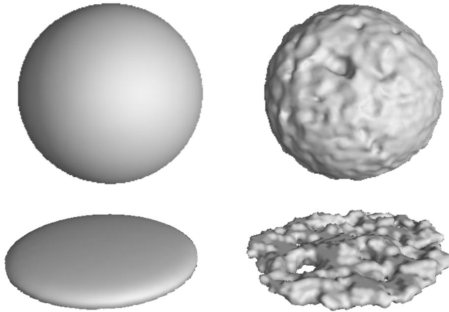
Fig. 3: 3D renderings of the studied pores, shown as solid bodies for better visualization. Top: Spherical pore ( $d=3\text{mm}$ ), bottom: elliptical pore ( $3\text{mm}/0.6\text{mm}$ ). Left: Idealized pore shape. Right: Real pores in additively manufactured parts. Surface segmented from CT images
