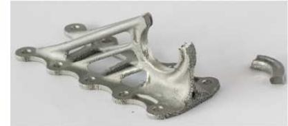
Notch, specimen 2 of 3, HS<sub>1</sub> and HS<sub>2</sub>
