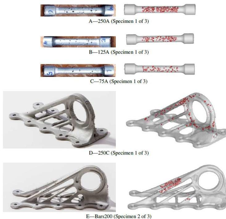
Figure 1: Five out of 36 test specimens. A–C: Tension rods, D–E: Aeronautic parts. For each specimen: Left—photograph, before destructive test. Right—CT image data of same specimen, outer surface transparent, porosity highlighted in red. [1]
