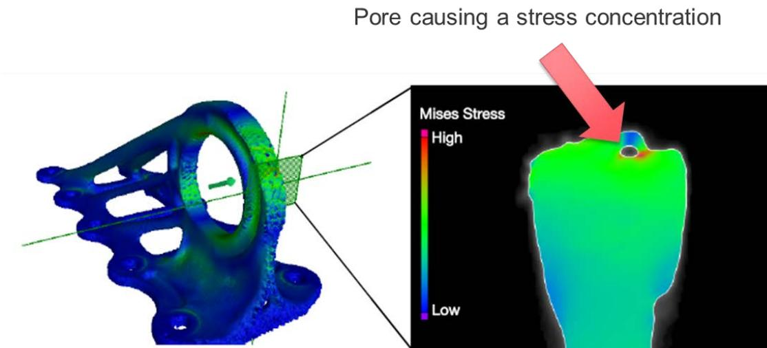
Figure 3: Simulated stress distribution in a 3D printed component under a static load, showing a pronounced stress concentration around a pore close to the surface
