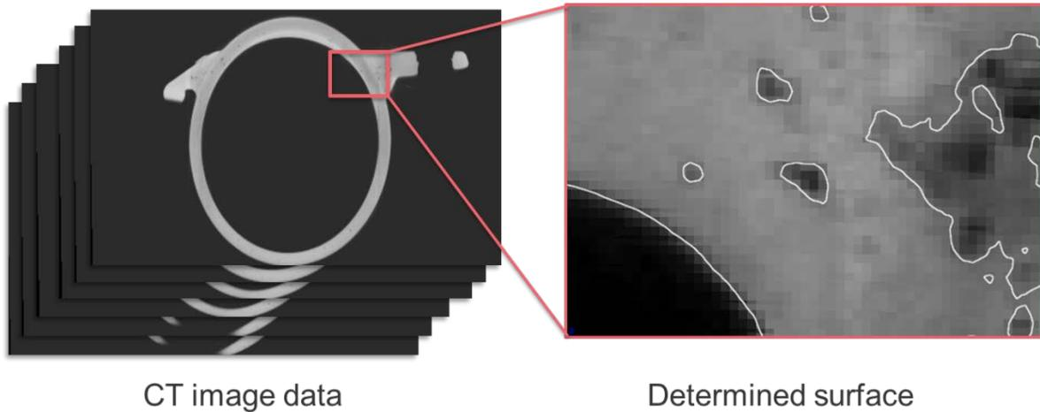
Figure 2: Example of a CT scan of a component with pores. Left: Stack of 2D slice views. Right: External and internal surfaces determined with sub-voxel accuracy
