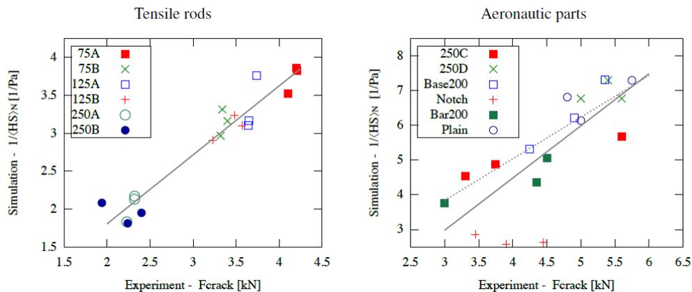
Figure 4. Measured force at first crack ( $F_{\text{crack}}$ ) versus prediction from simulation ( $1/\langle HS \rangle_N$ ). Each data point represents one tested specimen. Left—tensile rods; right—aeronautical parts. The straight line is a least-squares fit to the data. Dotted line: least-squares fit without the notch-type porosity pattern [3]
