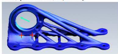
Notch, specimen 2 of 3, HS 1 and HS 2
