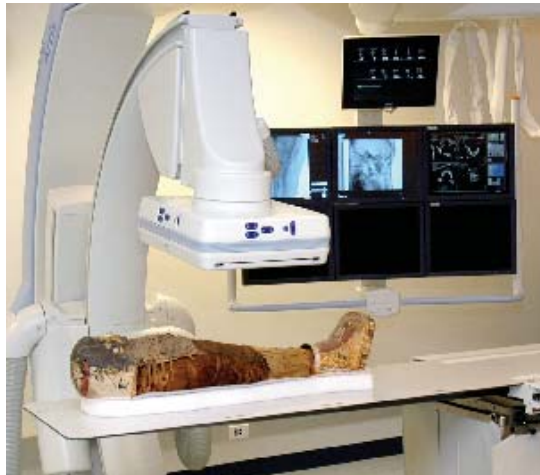
The Mummy on C-Arm Axiom Scanner at Stanford. Cross sectional slices as small as 200 microns were captured with this system.
